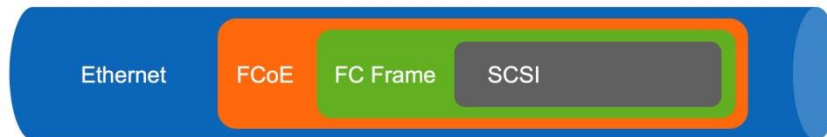
Figure 1) FCoE is the encapsulation of Fibre Channel into Ethernet.
